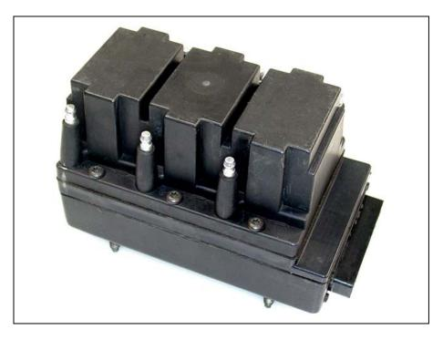
Since the CCCI Simulator is designed to test the 1986 thru 1989 turbo CCCI coil packs, you will need this adapter to change the gender and positions of key wiring between the different years. The adapter attaches between the CCCI Simulator and the coil module.
