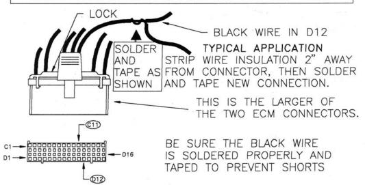
SOLDER THE BLACK WIRE OF THE NEW MAT SENSOR WIRING TO THE BLACK WIRE IN LOCATION D12 AS SHOWN. REMOVE THE TERMINAL LOCK ON THE "C" SIDE AND INSERT THE TERMINAL OF THE BROWN WIRE INTO LOCATION C11.
