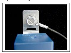
Run the positive feed wire over to the battery and attach to the positive lug. If your battery is in the trunk, you should attach this ring terminal to the battery junction box (if used) or on the starter positive stud. If attaching to the starter stud, be sure all wiring is permanently positioned out of the way of the hot exhaust components.
