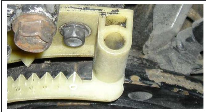
This timing window is (of course) buried in the front of the engine and is difficult to see. Once you detect compression pressure, the notch on the harmonic balancer (which rotates clockwise) will have approached the "0" timing mark and probably passed it up. You will likely need to grab a hold of the serpentine belt and rotate the belt pulley counter-clockwise slightly to re-align the timing notch so that it is in alignment with the "0" timing mark as shown here:
