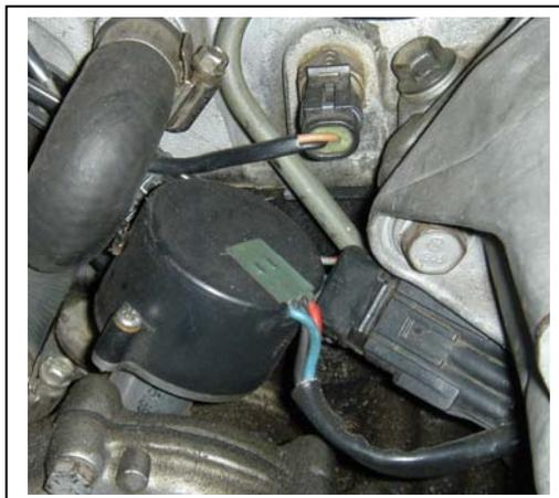
This position is typical of a factory installed cam sensor, and is exactly how GM had installed the sensor from the beginning. If you remove the two Philips screws and unplug the connector, you will see the interrupter ring directly under the cap, as shown here.
