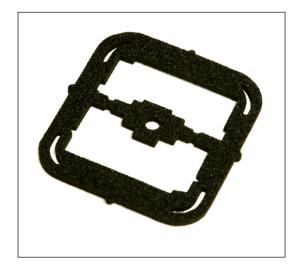
The Fuse Panel is fastened to the backside of the C100 connector and is held in place with two long screws. Working under the dash, remove the hardware that secures the connector to the firewall. Pull the bulkhead away from the firewall to expose the face end of the connector. You will find the original gasket at the base of this connector face.
