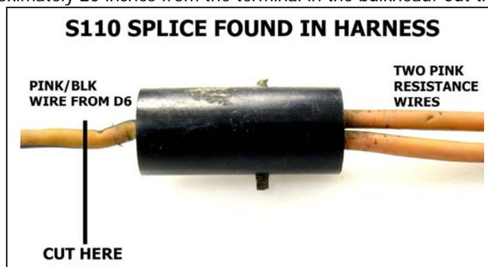
At this point, you will have removed both of the resistance wires and the splice. You will have remaining approximately 18 inches of pink/black stripe wire between the CCCI module connector, cavity "P"...
