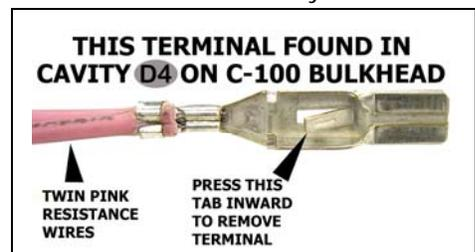
Next, insert the new terminal provided in this kit into the D6 cavity. Re-install the locking comb once the terminal is seated. The new terminal has 20 inches of new copper wire along with a butt-splice attached to the opposite end. Peel back 24 in. of the conduit and tape between the C-100 bulkhead and the CCCI module connector. You will find the molded S110 wire splice approximately 20 inches from the terminal in the bulkhead. Cut the resistance wires and molded splice as shown here:
