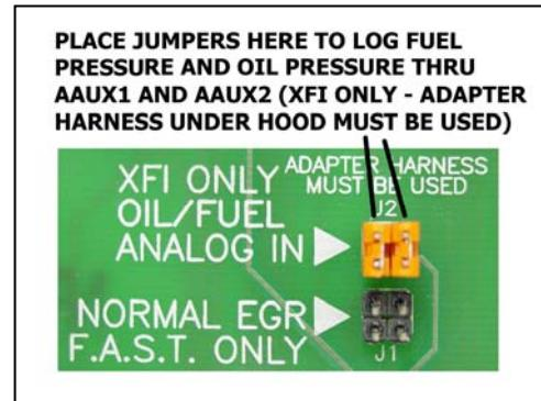
The jumpers are installed at the factory in their "NORMAL EGR" position as shown in the image on the left. To use the pressure logging function, you will need to remove the jumpers and relocate them as shown in the image on the right. Additionally, there is an internal relay on the PC board that interfaces with the external fuel pump relay. This relay provides the correct interface between the ECU and your factory fuel pump relay.
