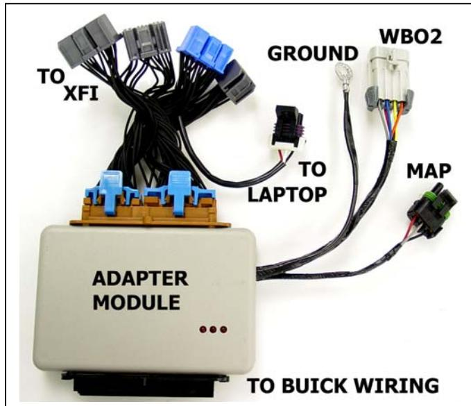
**NOTE:** MAP Sensor must be plugged into the MAP connector found on this adapter. Optionally, you can use an adapter, Caspers PN 108119 shown below which plugs into the GN's C437 connector under the dash and allows use of a 3-bar MAP sensor to be used in place of the OEM 2-bar sensor, in the stock factory location.
