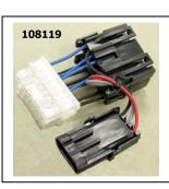
**NOTE:** MAP Sensor must be plugged into the MAP connector found on this adapter. Optionally, you can use an adapter, Caspers PN 108119 shown below which plugs into the GN's C437 connector under the dash and allows use of a 3-bar MAP sensor to be used in place of the OEM 2-bar sensor, in the stock factory location.
