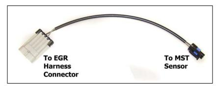
Use the MST harness, included in kit, to connect MST sensor to ECU via the unused EGR connection. Note there are two wires on the EGR connection which have been re-routed to the DFI ECU, to serve as the manifold temperature input. Using this harness properly connects the sensor to the ECU.
