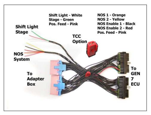
Note that there are two pigtails and a free-hanging red connector on the extension. The pigtails are for optional NOS control, and optional Staging and Shift Light functions. Connect to these pigtails as needed, outlined in the DFI installation instructions. The red JUMPER connector will be used when the TCC Lockup option is installed.
