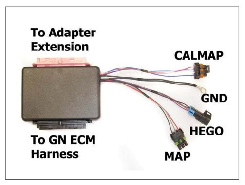
To connect the adapter box to the GEN 7 DFI system, an 8 inch extension is used:
