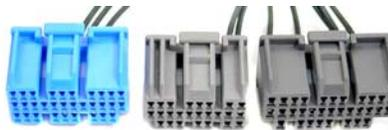
These A, B, and C plugs attach to XFI ECU only.
