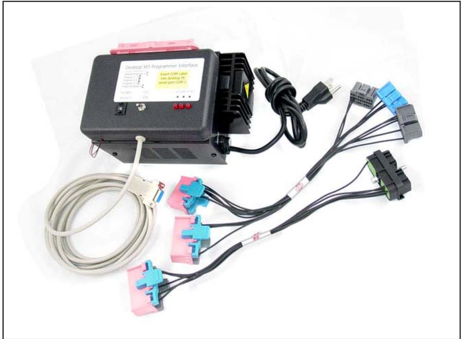
To program the ECU, plug all connections in securely. Insert AC plug into 115VAC grounded outlet. Be sure the data connection is recognized by your host PC and you are running the current OEM software. Be sure the main power switch (at the base of the power supply) is turned on. The STBY LED must be illuminated.
