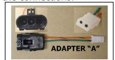
This Dead-End Connector externally bypasses the following wiring of the CCCI ignition system connector to permit use of a distributor:
